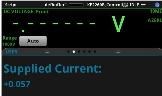
7. Selecting **Output ON/OFF** will cause the state of the instrument's source output to change either ON or OFF depending on the current state.
