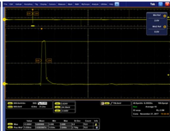
1 These pulses represent the Write1 pulse, also known as the Set Pulse. 1 ns pulse width is shown here, as well as a 200 ps pulse width to show the AWG capabilities.
