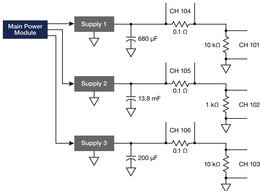
Figure 3. Test circuit for monitoring the turn-off DC current of an energy storage system
