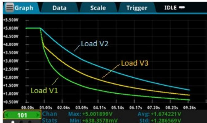
Figure 8. Collective plot of voltage drops across loads
