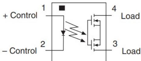
Figure 2. Simple solid-state relay.
