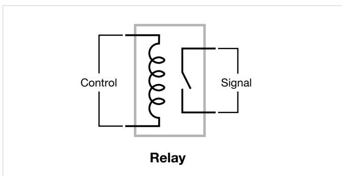
Figure 1. Simple electromechanical relay.
