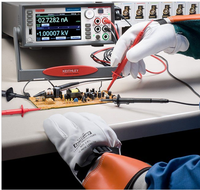
Figure 5: Using proper safety gloves when working with high voltages on energized components.
