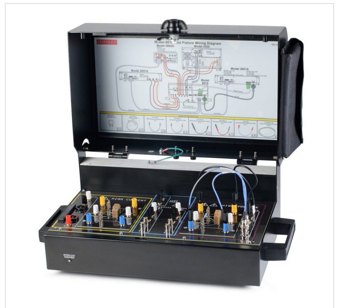
Figure 3: Properly grounded testing fixture
