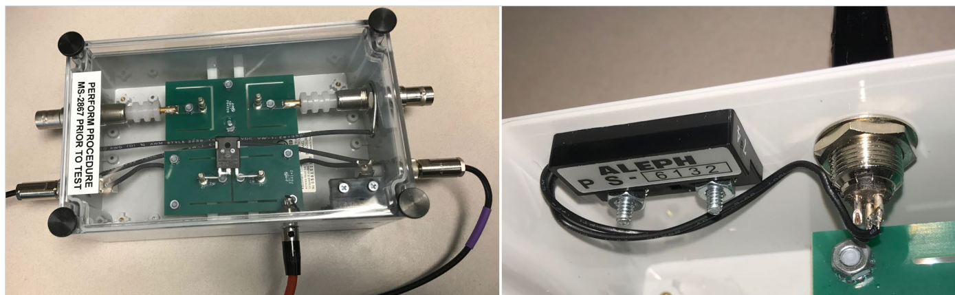
Figure 7. Test Fixture for testing the high voltage diode which includes a safety interlock relay system.
