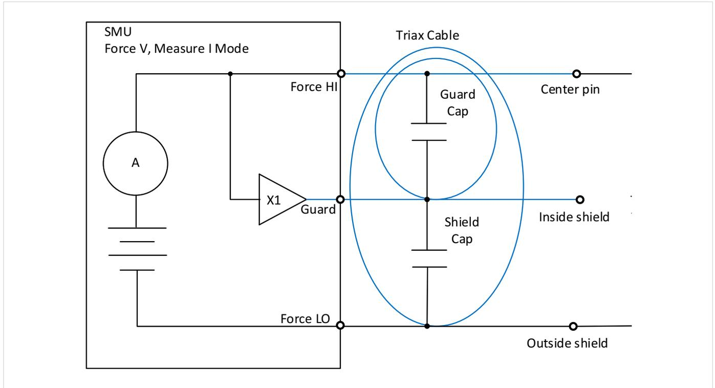
FIGURE 2. Illustration of guard, shield, and load capacitances.
