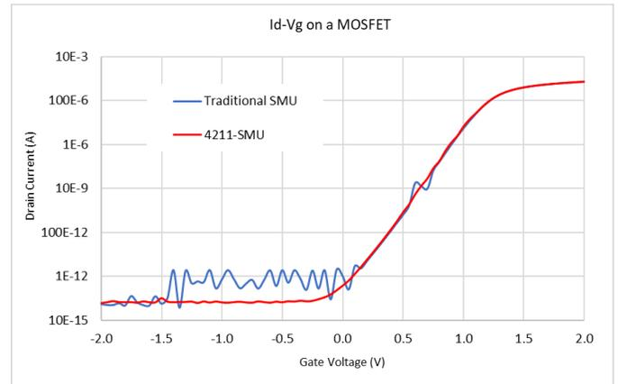
**FIGURE 8.** nMOSFET  $I_d$ - $V_g$  curves generated using both traditional SMUs and 4211-SMUs using 20 m triax cables.
