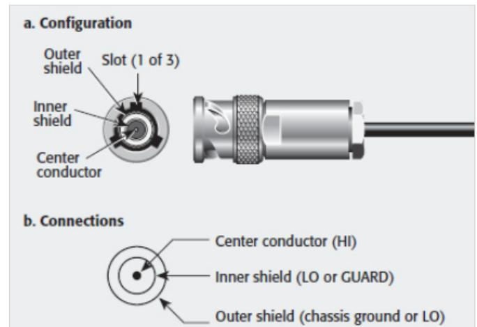
FIGURE 1. Configuration of a triaxial connector.
