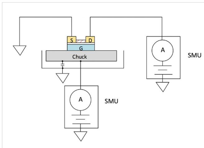
FIGURE 11. Using two SMUs to test a nano-FET.
