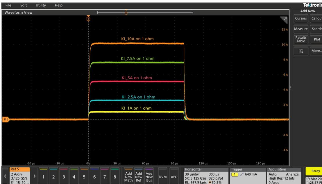
Figure 7: 2601B-PULSE 100 μs amplitude sweep at 1, 2.5, 5, 7.5, and 10 A.
