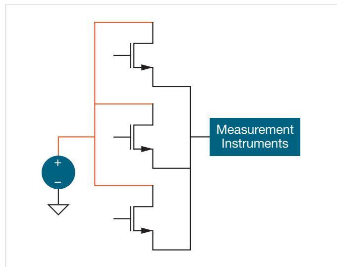
Figure 1: Parallel devices connected to a power supply.
