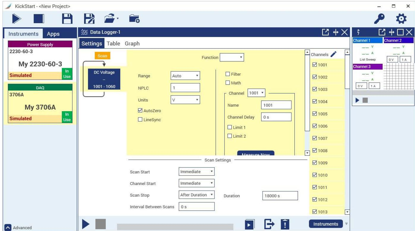
Figure 5: Configuring the 3706A System Switch / Multimeter using the Data Logger App in KickStart Software.
