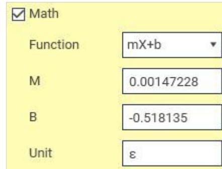
Figure 5: Applying math coefficients and user-specified units.
