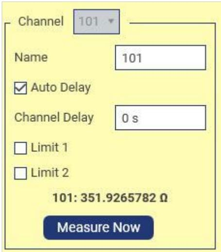
Figure 4: Measuring the device in its unstrained state will give us one of our known factors to be used in computing strain.
