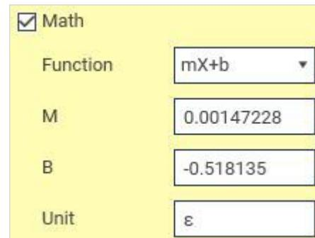
Figure 5: Applying math coefficients and user-specified units.
