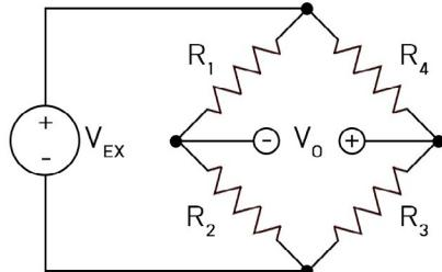
Figure 1: Wheatstone bridge configuration for use in strain measurement.
