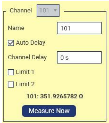
Figure 4: Measuring the device in its unstrained state will give us one of our known factors to be used in computing strain.
