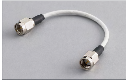
CA-451A: 10.8 cm (4.25 in) RG188 coax cable terminated with an SMA male plug on each, 50 \Omega impedance.
