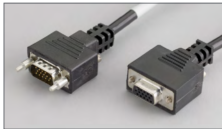
4200-RPC-2: Remote PreAmp cable terminated at each end with a high density DB15 connector. This cable connects a 4200-SMU or 4210-SMU source measurement unit installed in a 4200A-SCS to a remotely mounted 4200-PA PreAmp. 2 m (6.5 ft) (one included with each 4200-PA).
