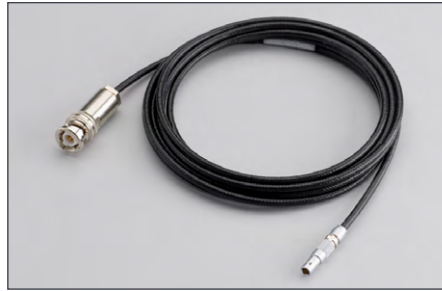
4200-MTRX-*: Ultra low noise SMU triax cable is terminated with a miniature male triax connector on one end and a standard 3-slot male triax connector on the other end. This cable connects a 4200-SMU or 4210-SMU source measurement unit installed in a 4200A-SCS to a test fixture. (4200-MTRX-* cables are intended only for connection to an SMU that does not have a 4200-PA PreAmp installed.)
