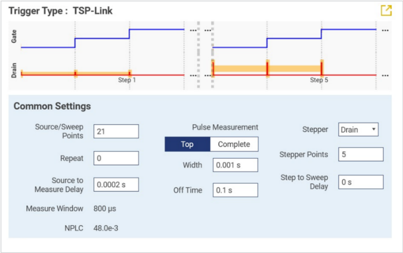
Figure 5. Pulse Setting for On-State Resistance.
