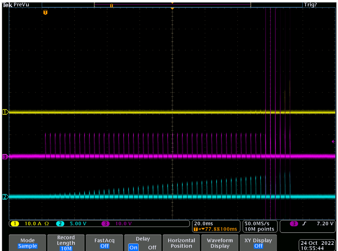
Figure 6. Oscilloscope waveforms of the Vg-Id test (yellow - drain I, magenta - drain V, blue - gate V).
