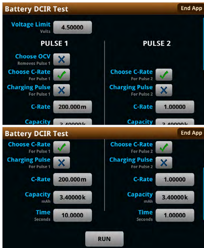
Figure 8: DCIR test settings for the Ultralast 3400 mAh 18650 cell.
