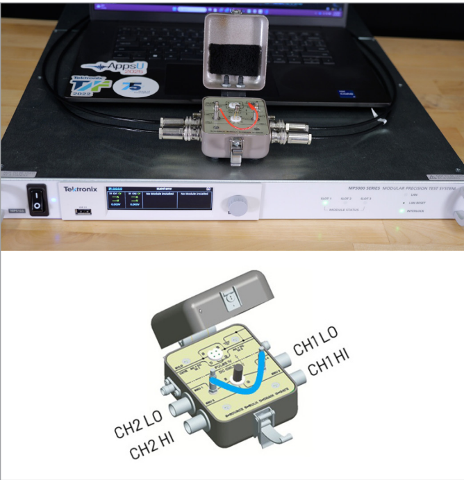
Figure 13: An SD210 N-Channel MOSFET installed in an 8101-PIV Test Fixture connected to an MP5000 SMU Module via Triaxial Cables
