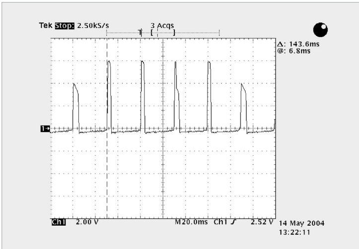
FIGURE 3-25: Unstable Measurement of 200 H Inductor
