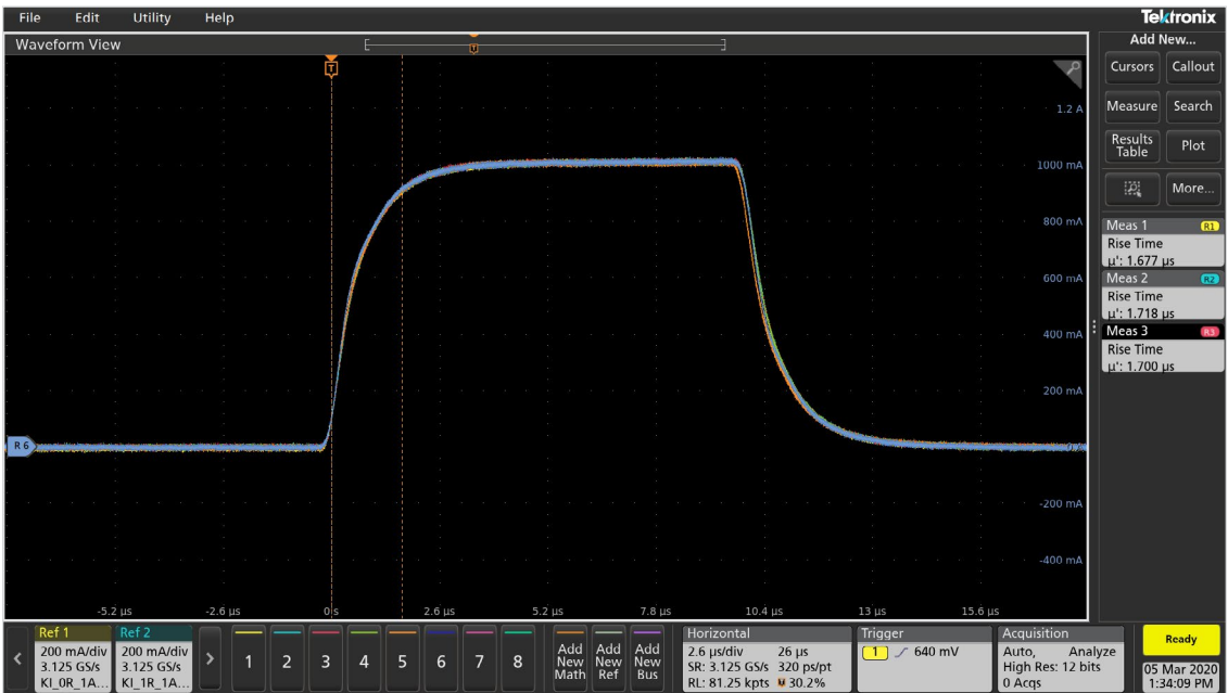
Figure 14. 2601B-PULSE 1 A pulse on 1, 2.5, 5, 7.5, and 10 ohm resistors.
