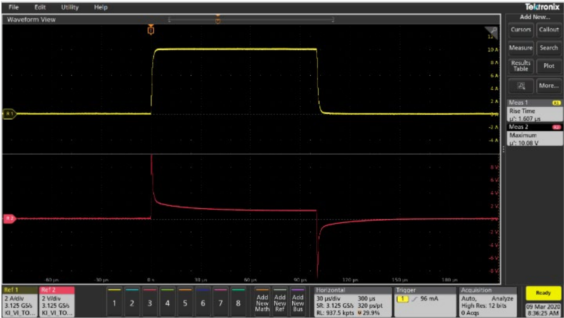
Figure 6. 1.6 \mu s rise time 10 A pulse on inductor 1 \mu H.
