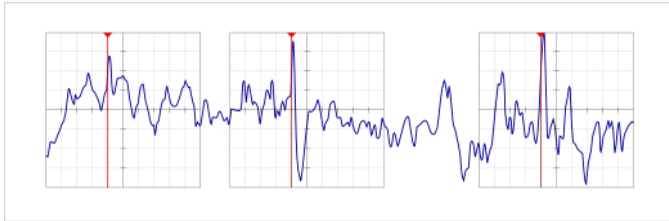
Figure 4: Triggered datalogging will have gaps in the captured data. The red vertical line indicates the trigger point.
