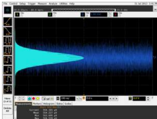
BW set to 33 GHz using standard acquisition shows 554uV RMS noise
