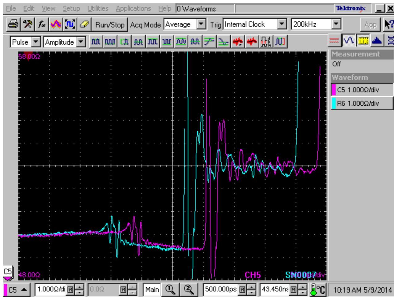
TDR of a single ended test coupon using a P8018 probe.
