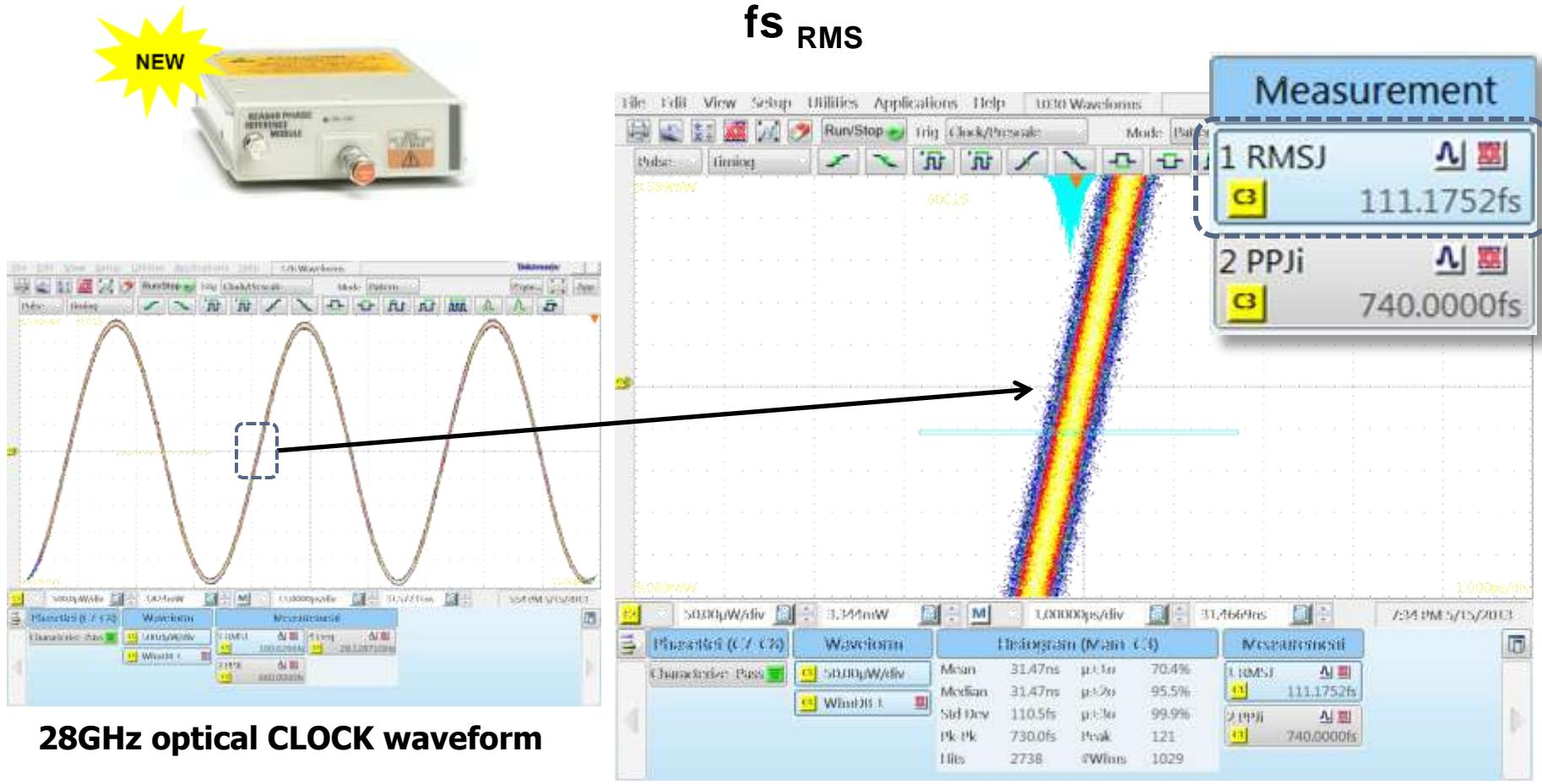
28GHz optical CLOCK waveform
