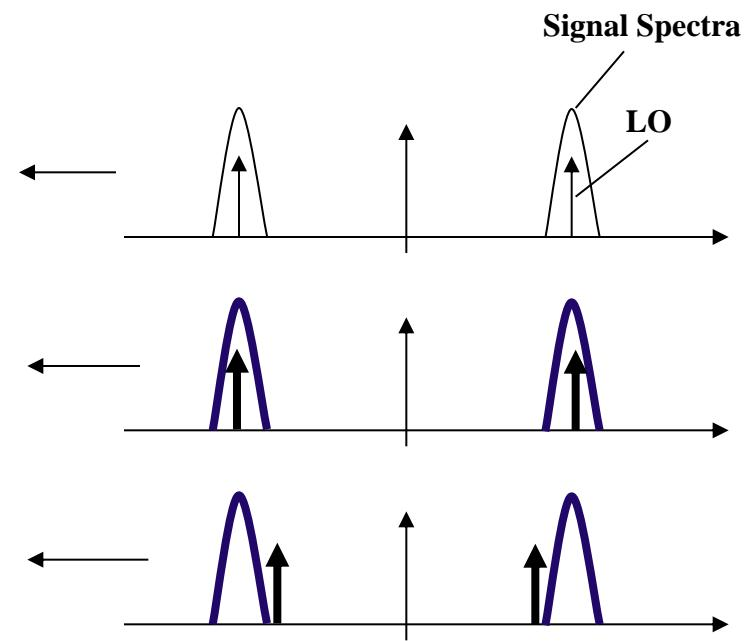
Without PLL, frequency and phase error must be corrected in DSP
