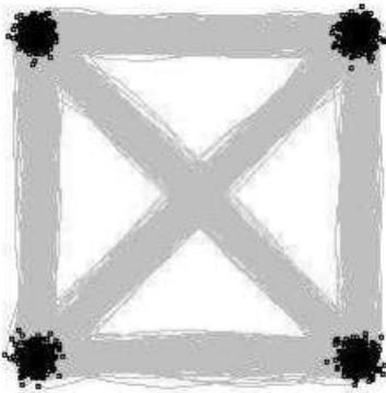
Figure 2 – IQ diagram for the same QPSK coding
