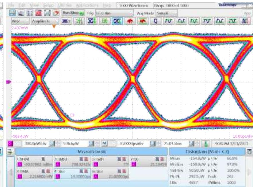
Signal source : 1550nm MZM Tx at 0dBm, 25.78125 Gb/s, PRBS31
