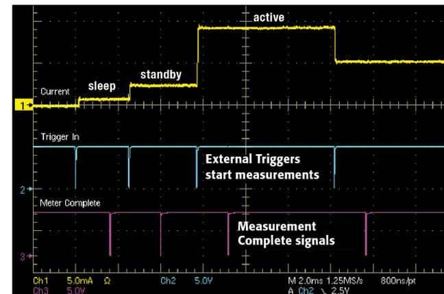
Series 2280S power supplies measure the start-up load currents as a device powers up. An external trigger tells the Series 2280S when to make a measurement. The Series 2280S signals when the measurement is completed so that the device can be put in its next state.
