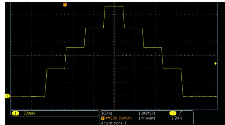
**List Mode** automatically steps the voltage through the programmed steps. With the Series 2280S supplies, the output can be displayed using the internal graphing capability.
