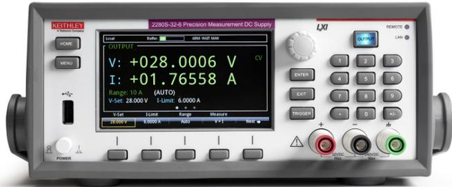
Keithley's Series 2280S Precision Measurement, Low Noise, Programmable DC Power Supplies can source stable, low noise voltages as well as monitor load currents over a wide dynamic range from amps to 100 nanoamps. The Model 2280S-32-6 can output up to 32V at up to 6A; the Model 2280S-60-3 can output up to 60V at up to 3.2A.
