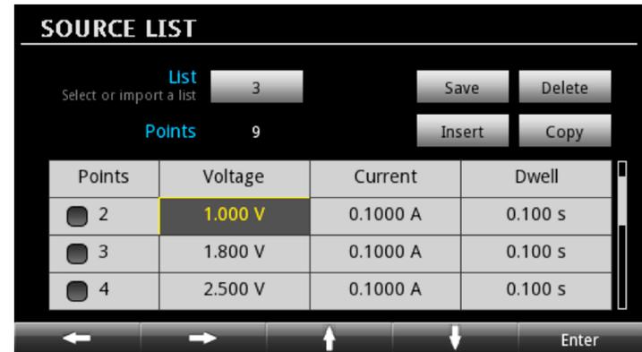
Create a test consisting of a number of output voltage levels using the Series 2280S' **List Mode** setup screen. Alternatively, download a list using a USB flash drive.
