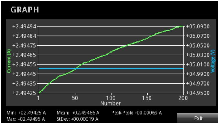
Use the Series 2280S' built-in graphing capability to monitor load current. Up to 2,500 data points can be stored, and statistics on the data can be automatically displayed on the graph for a quick and easy analysis of the results.
