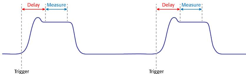
Series 2280S power supplies enable time-critical measurements on fast-changing or pulse-like loads. An external trigger initiates the acquisition. Programmable delay and measure times enable measurements at a specific time on the load current pulse such as when the peak has stabilized.
