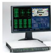
A unique method for configuring a variety of different views of the video signal within four tiles. This display technology is called FlexVu™ and allows the user to customize their measurement
