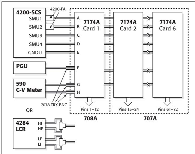
Figure 6. Semiconductor characterization system diagram.
