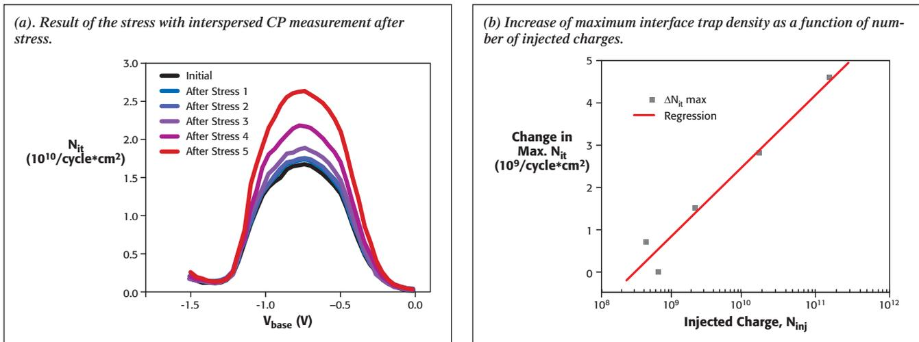
Figure 5. Stress and charge-pumping measurement on a nMOSFET transistor with an ALD  $\text{HfO}_2$  gate dielectric and chemical oxide interfacial layer.
