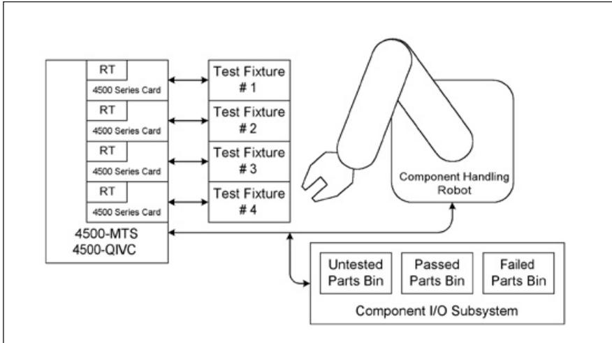
Figure 4: In this example of synchronous concurrent testing a robot component handler tends a four-site test system. The robot loads modules in each test head in turn, triggering test equipment as it does so.
