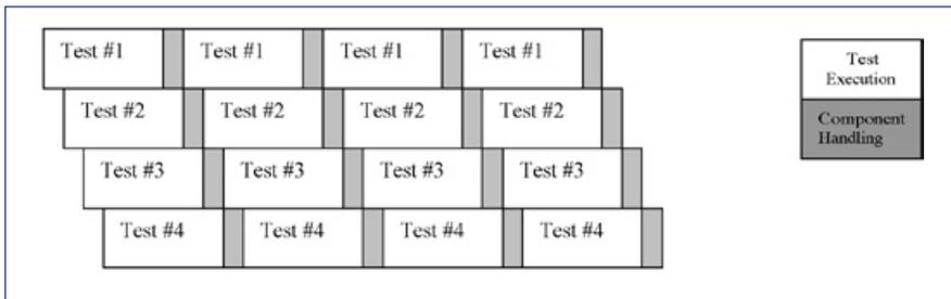
Figure 5: Synchronous concurrent test sequencing nearly quadruples throughput compared to serial test.
