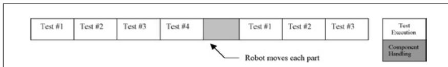
*Figure 2: Multiplex test can double throughput when the multiplexer operation is much faster than the component handler operation.*
