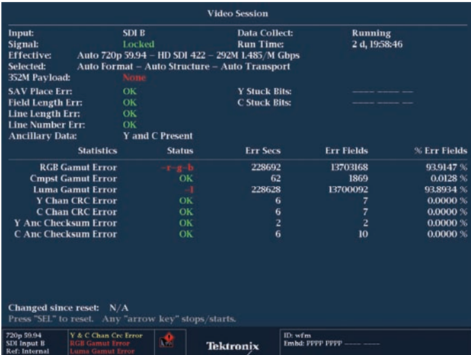
Figure 3. Status display showing CRC errors of an HD SDI signal.
