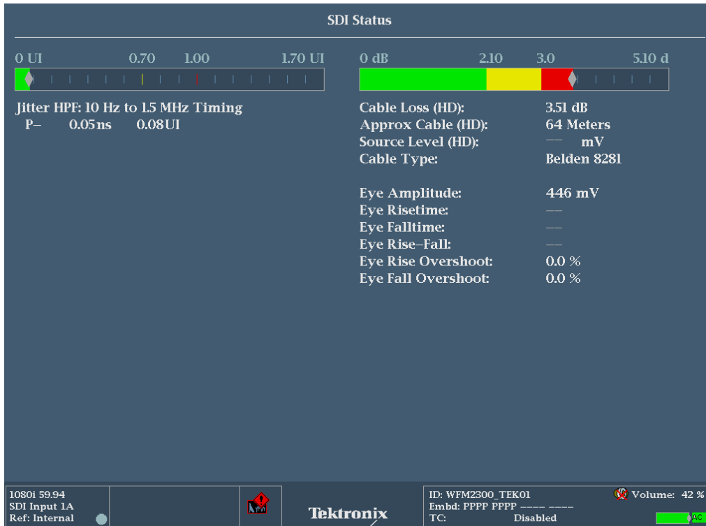
Figure 3. SDI Status Display showing physical layer measurement summary.
