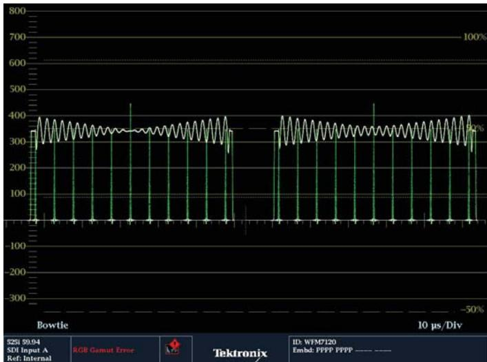
Figure 96. Bowtie display Pr gain error vs. Y.
