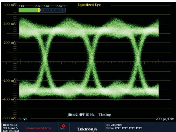
Figure 83. Unterminated Eye display on the WFM7120.
