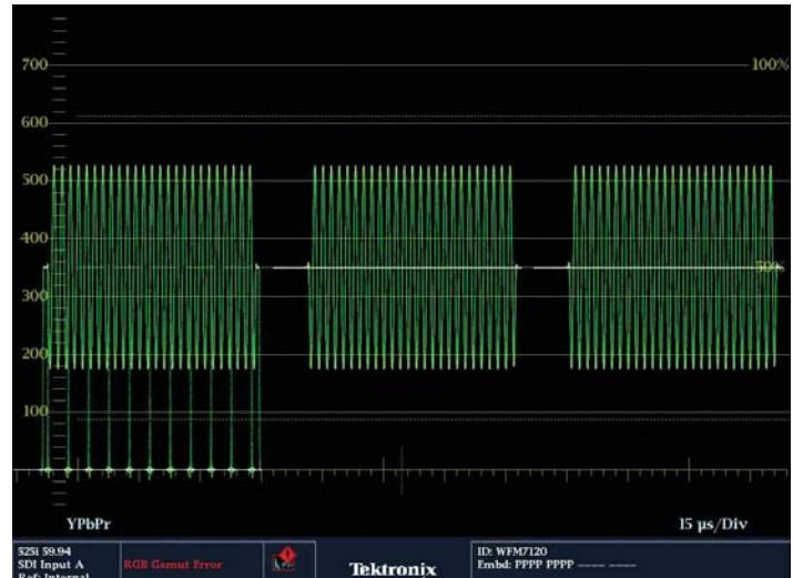
Figure 93. Bowtie test signal.
