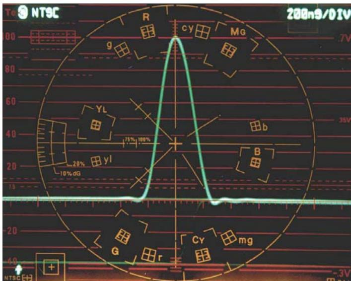
Figure 75. Correct 2T pulse, 1H MAG display.
