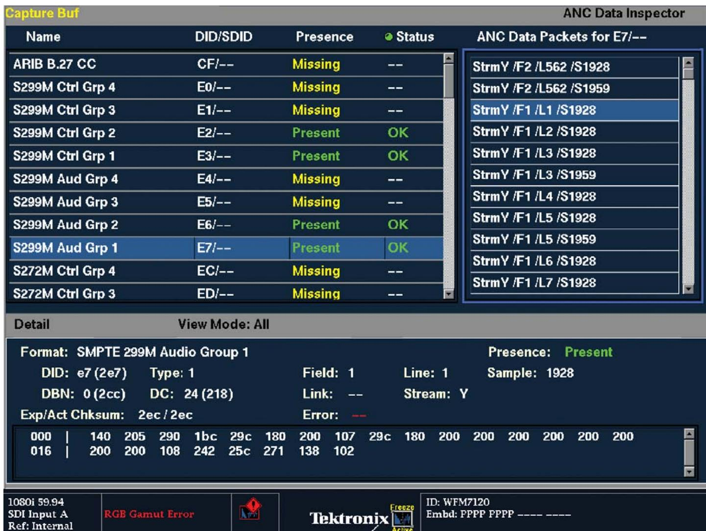
Figure 66. Capture Buffer display using Ancillary Data Inspector.
