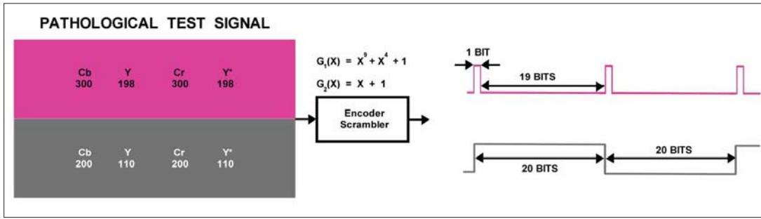
Figure 78. SDI Check Field "Pathological Test Signal."
