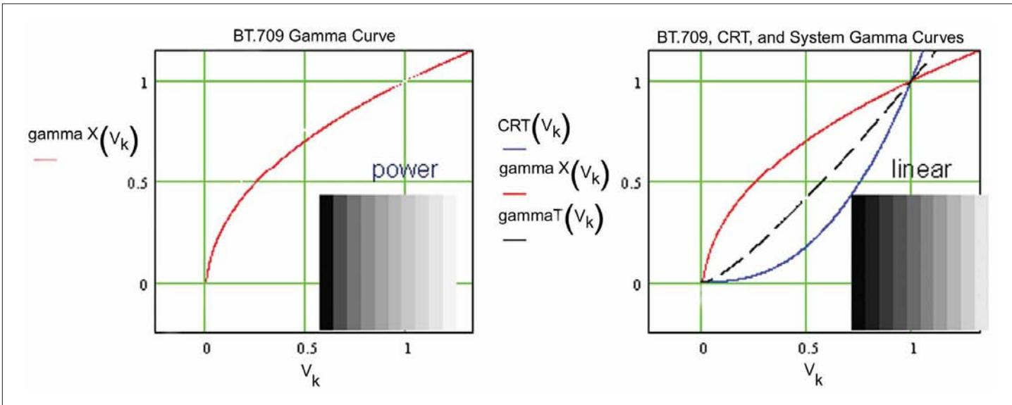
Figure 4. BT.709 gamma correction complements CRT display response.
