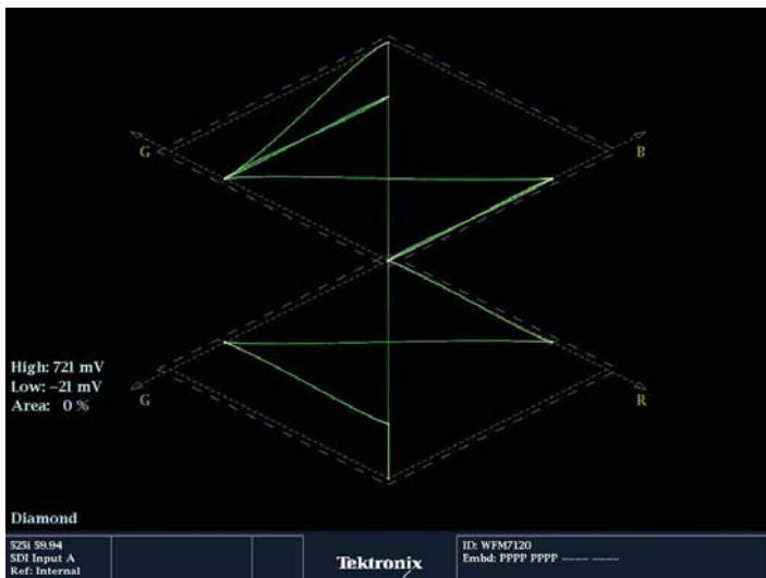
Figure 105. Tektronix Diamond display of 75% color bars.
