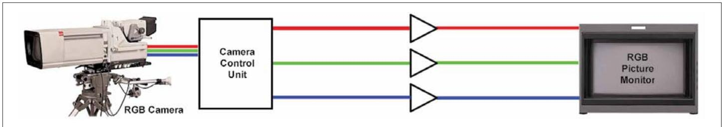
Figure 1. RGB from the camera with direct connections to the monitor.
