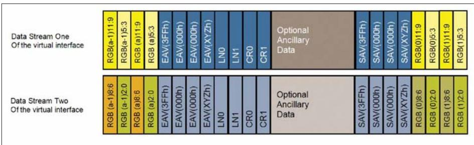
Figure 51. Level A R'G'B' mapping structure three.
