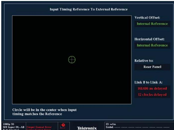
Figure 43. Inter-channel timing measurement of a Dual Link signal.
