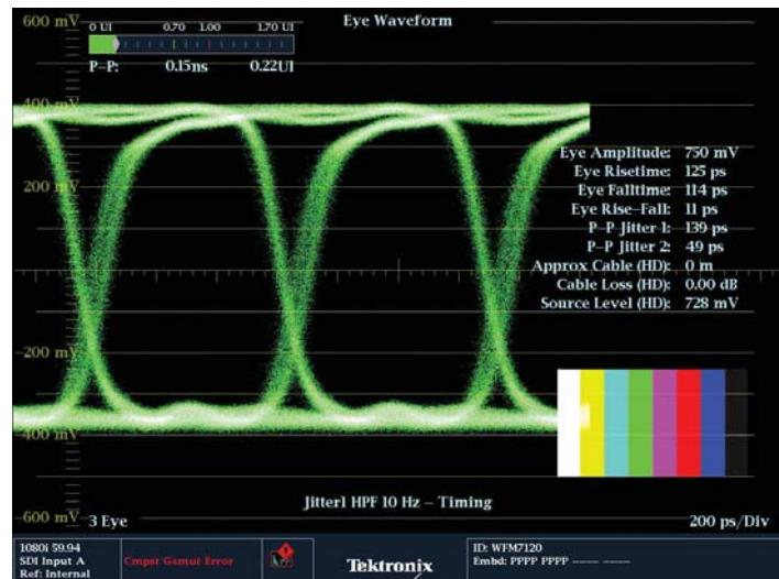
Figure 84. Non-symmetrical eye display on WFM7120.
