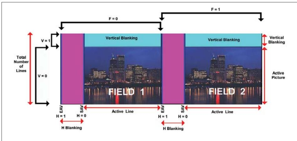
Figure 12. Layout of 2:1 interlaced digital frame.
