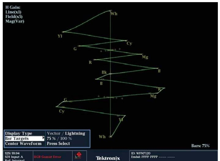
Figure 104. Lightning display with P'r gain error.
