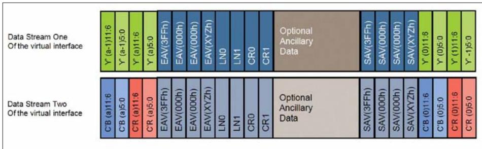
Figure 52. Level A Y'C'bC'r mapping structure four.
