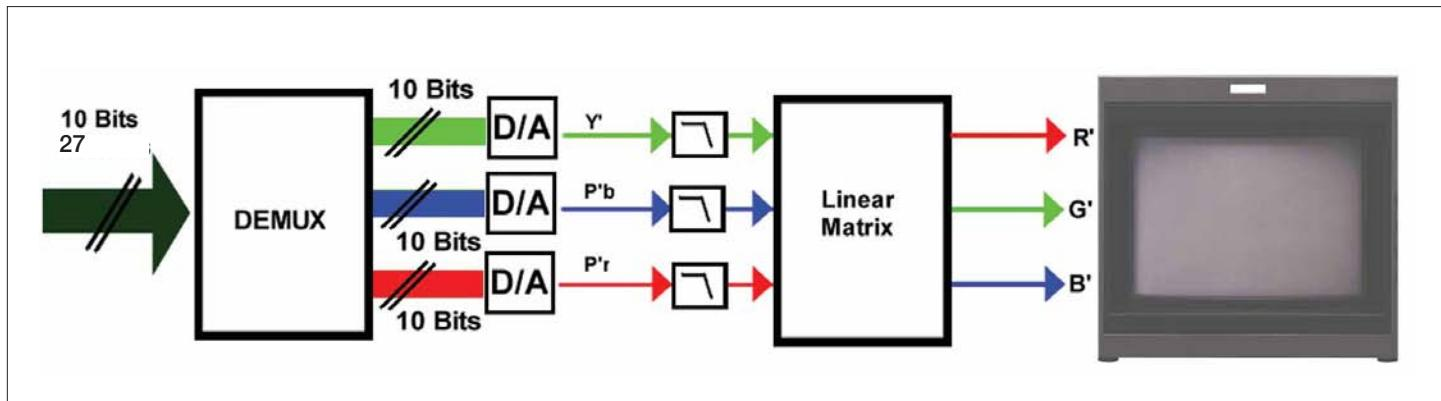
Figure 8. Recovering analog R'G'B' from parallel data.
