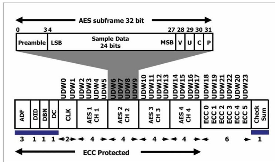
Figure 57. Structure of HD audio data packet.
