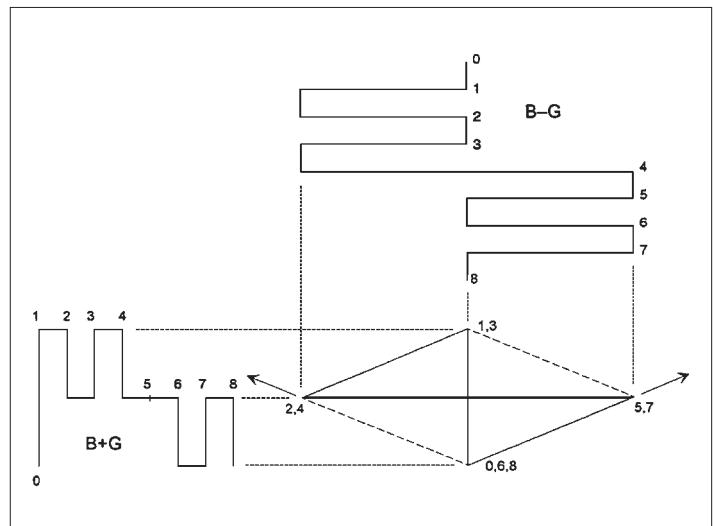
Figure 106. Development of the Diamond display, upper half.
