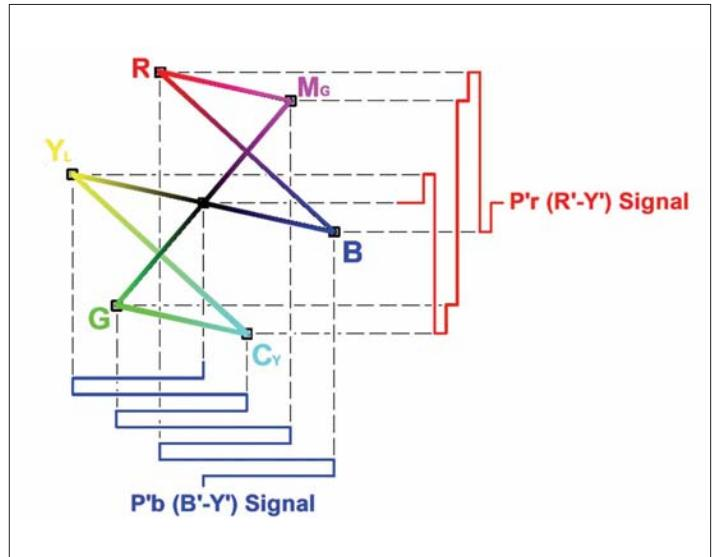
Figure 101. Development of the component vector display.
