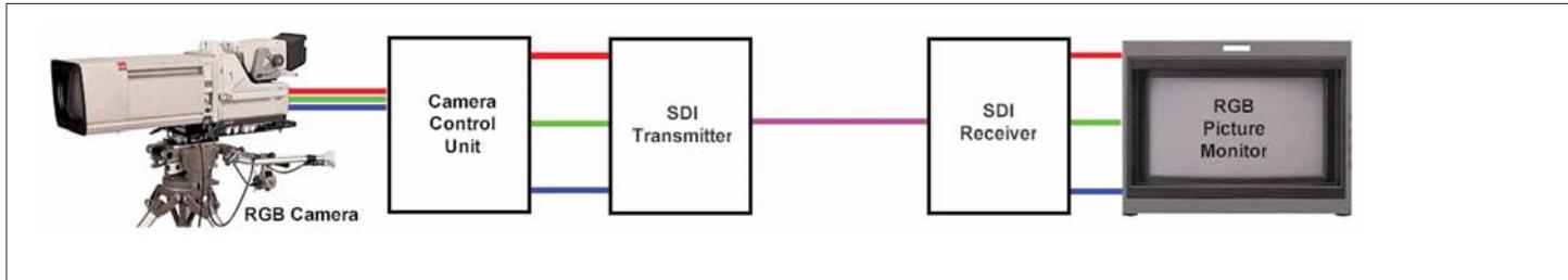
Figure 3. Digital transmission avoids analog signal degradation.
