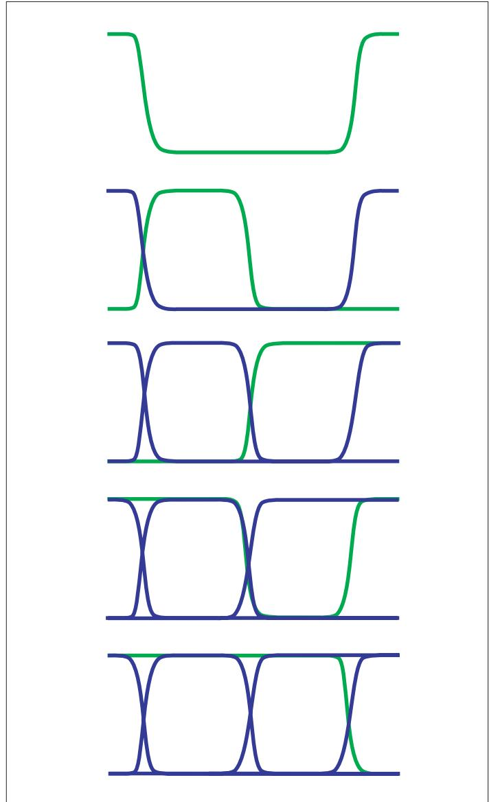
Figure 72. Development of the eye diagram.
