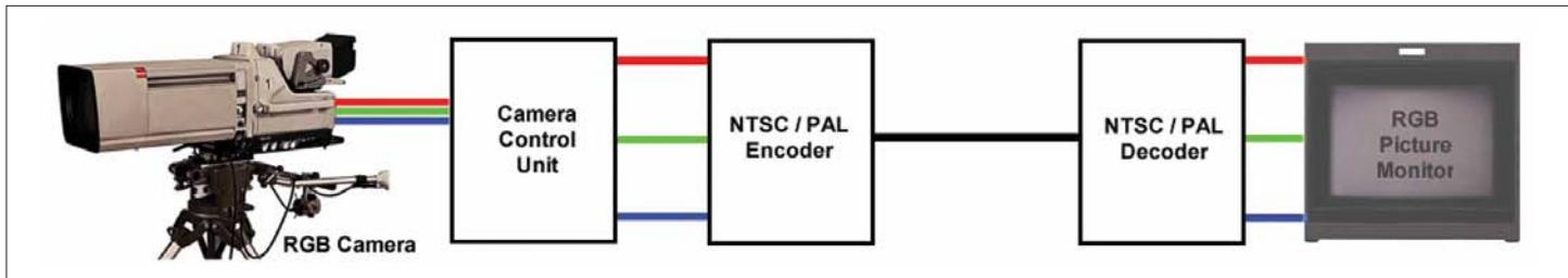
Figure 2. Video encoded to NTSC or PAL for transmission on a single coaxial cable.
