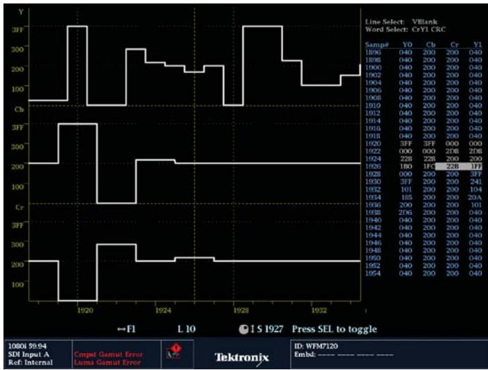
Figure 64. Data list display of the WFM7120 showing the ancillary data of a SMPTE352M packet.
