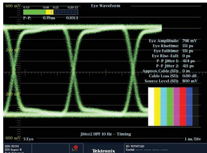
Figure 71. Correct 270 Mb/s data signal viewed with WFM7120.
