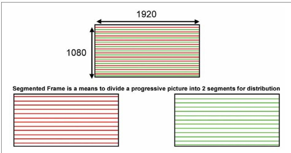
Figure 26. Conversion of a progressive frame into segments.
