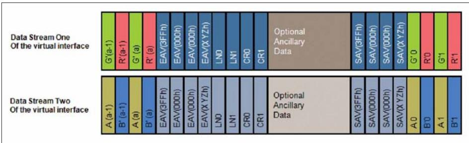
Figure 50. (Level A) R'G'B' mapping structure two.
