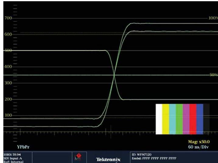
Figure 90. Interchannel timing measurement using green/magenta transition.
