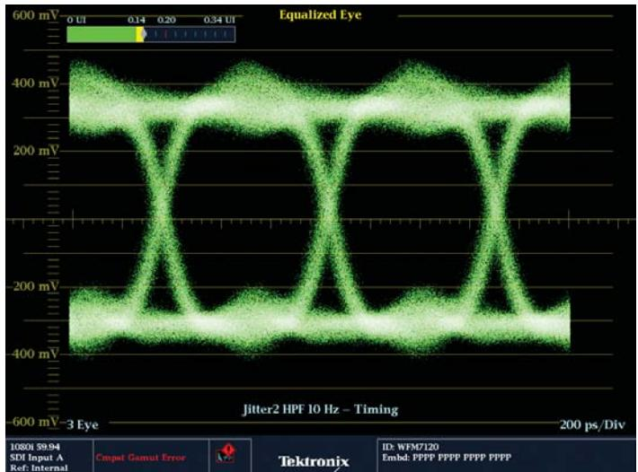
Figure 85. Equalized Eye mode on the WFM7120.
