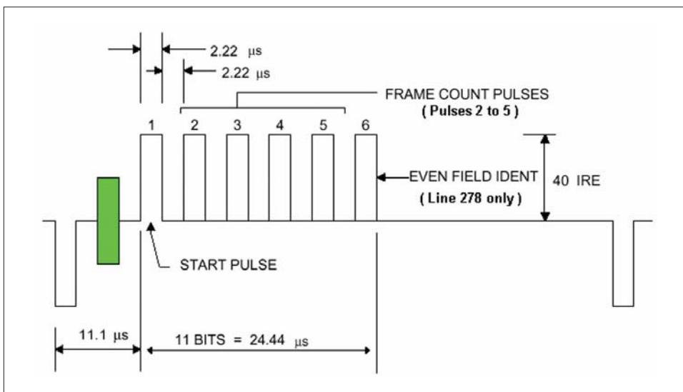
Figure 33. SMPTE 318M timing reference synchronizing line.
