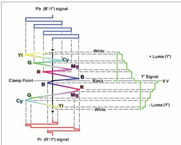
Figure 103. Development of the Tektronix Lightning display.
