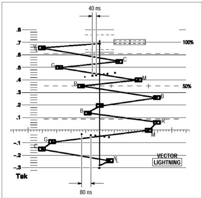
Figure 92. Lightning display for a 100% color bar signal.
