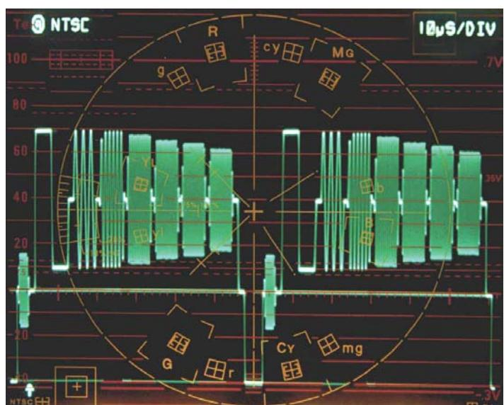
Figure 74. Multiburst with frequency response rolloff, 2H display.
