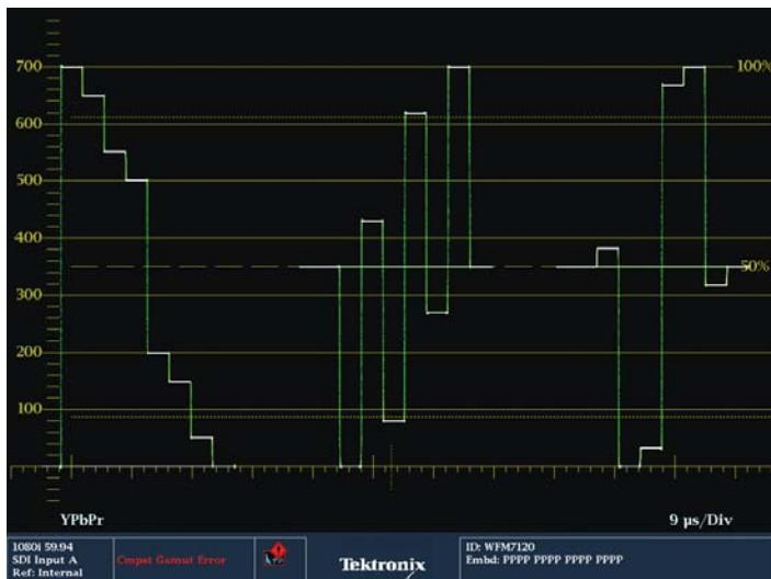
Figure 111. 100% color bar signal YPbPr for HD.
