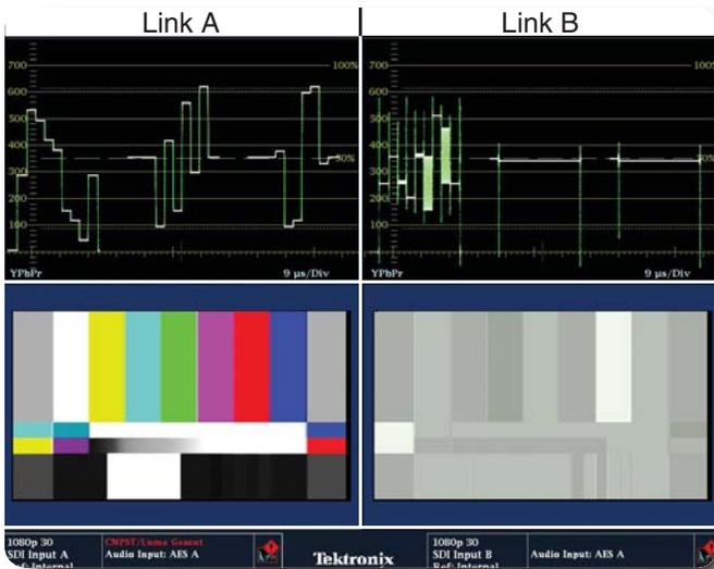
► **Figure 10.** Waveform displays of Dual Link A and B signals for Y'C'bC'r(A) 4:2:2:4 12-bit format.
