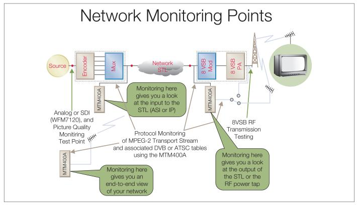
Figure 1. Multiple monitoring points throughout a broadcast network.
