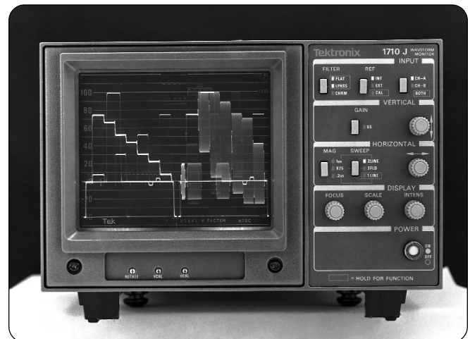
► Figure 2-2. The Tektronix 1710J NTSC Waveform Monitor displays video signals for amplitude and timing measurements.
