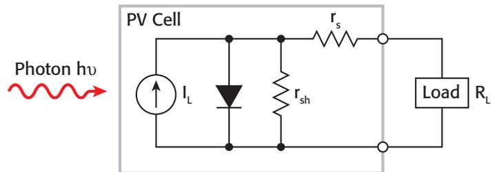
**Figure 1. Idealized equivalent circuit of a photovoltaic cell**
