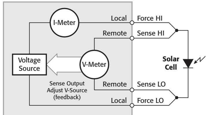
**Figure 4. Connections of 4200-SCS’s SMU to Solar Cell**
