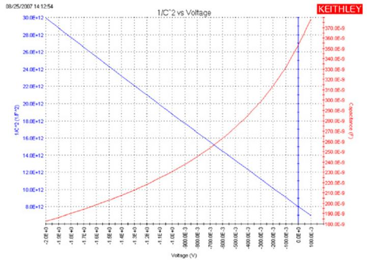
**Figure 12. 1/C<sup>2</sup> vs. Voltage of a Silicon Solar Cell**
