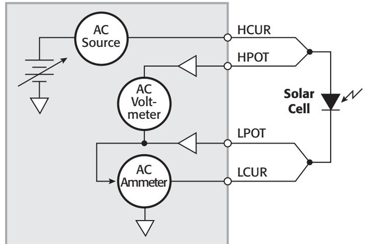
**Figure 10. Connecting the 4200-CVU to a Solar Cell**
