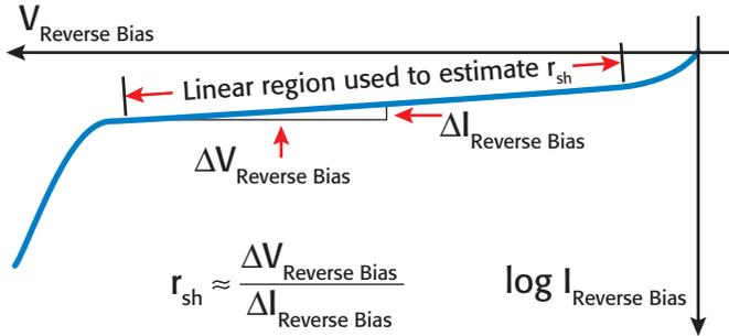
**Figure 8. Typical Reverse-Bias Characteristics of a PV Cell**
