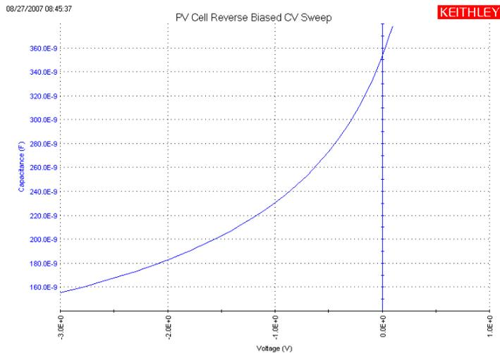
**Figure 11. C-V Sweep of Silicon Solar Cell**
