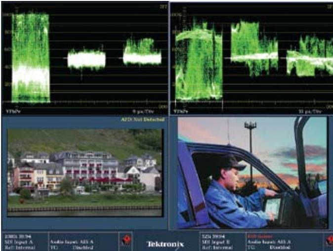
Figure 12. Simultaneous SD/HD Inputs using FlexVu™ display.
