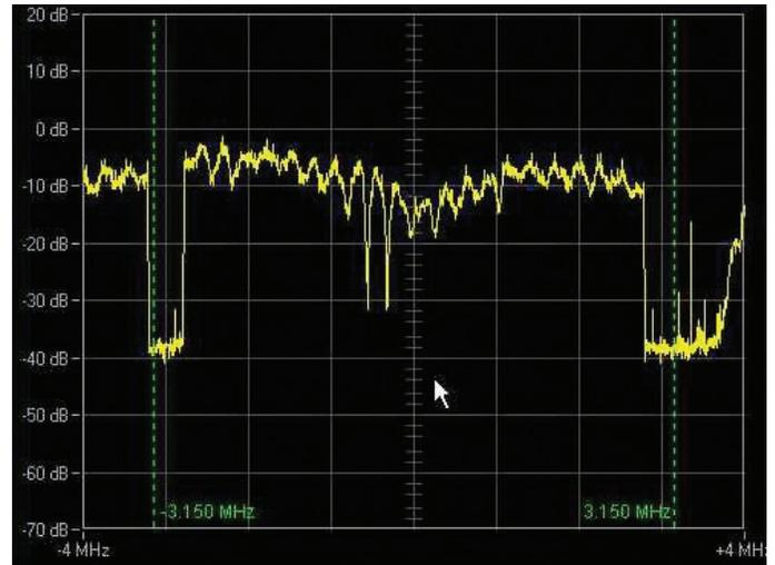
Figure 5. ISDB-Tb signal with poor frequency response. This signal has a digital carrier one channel below and a PAL signal one channel above.
