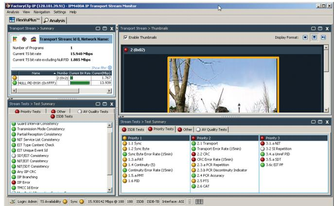
Figure 7. MTM400A measuring transport compliance from the ASI output of an RFM220.
