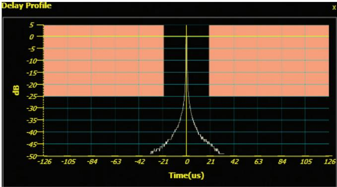
Figure 6. ISDB-Tb signal with no multipath or reflections.
