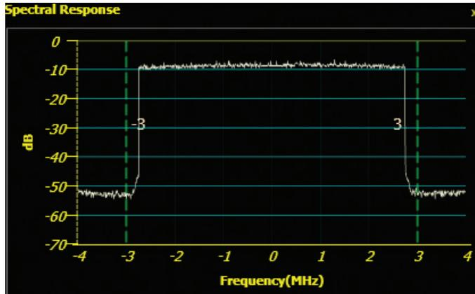
Figure 4. ISDB-Tb signal with good frequency response (no adjacent carriers).
