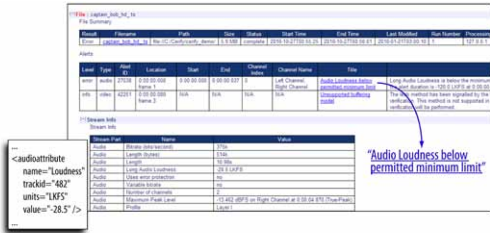
Figure 14. This report from the Tektronix Cerify automated QC solution has captured an audio error and documented all of its parameters.
