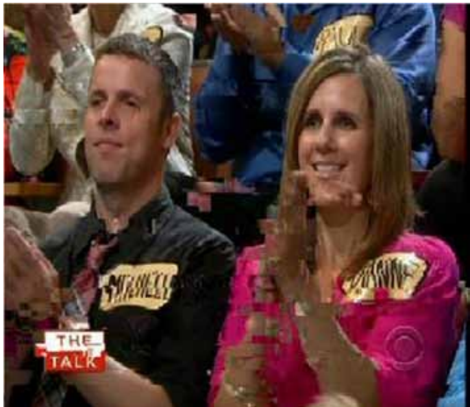
Figure 13. “Slice order” errors in MPEG transport streams can cause blockiness and other picture distortions.
