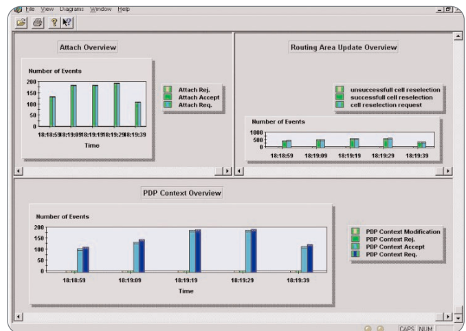
► Figure 3. The easy-to-read and effective graphical representation of sessions statistics available with Tektronix K1297-G20, allows technicians to easily diagnose processing problems.
