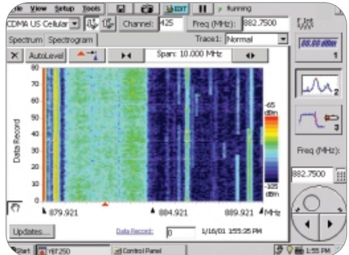
► **Figure 10.** Spectrogram of live cellular signals.
