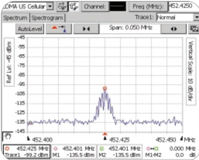
► **Figure 18.** Two-way radio with tone burst.
