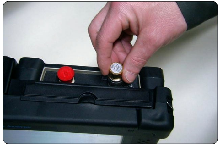
► Figure 16. Avoid improper attachment of the standard.
