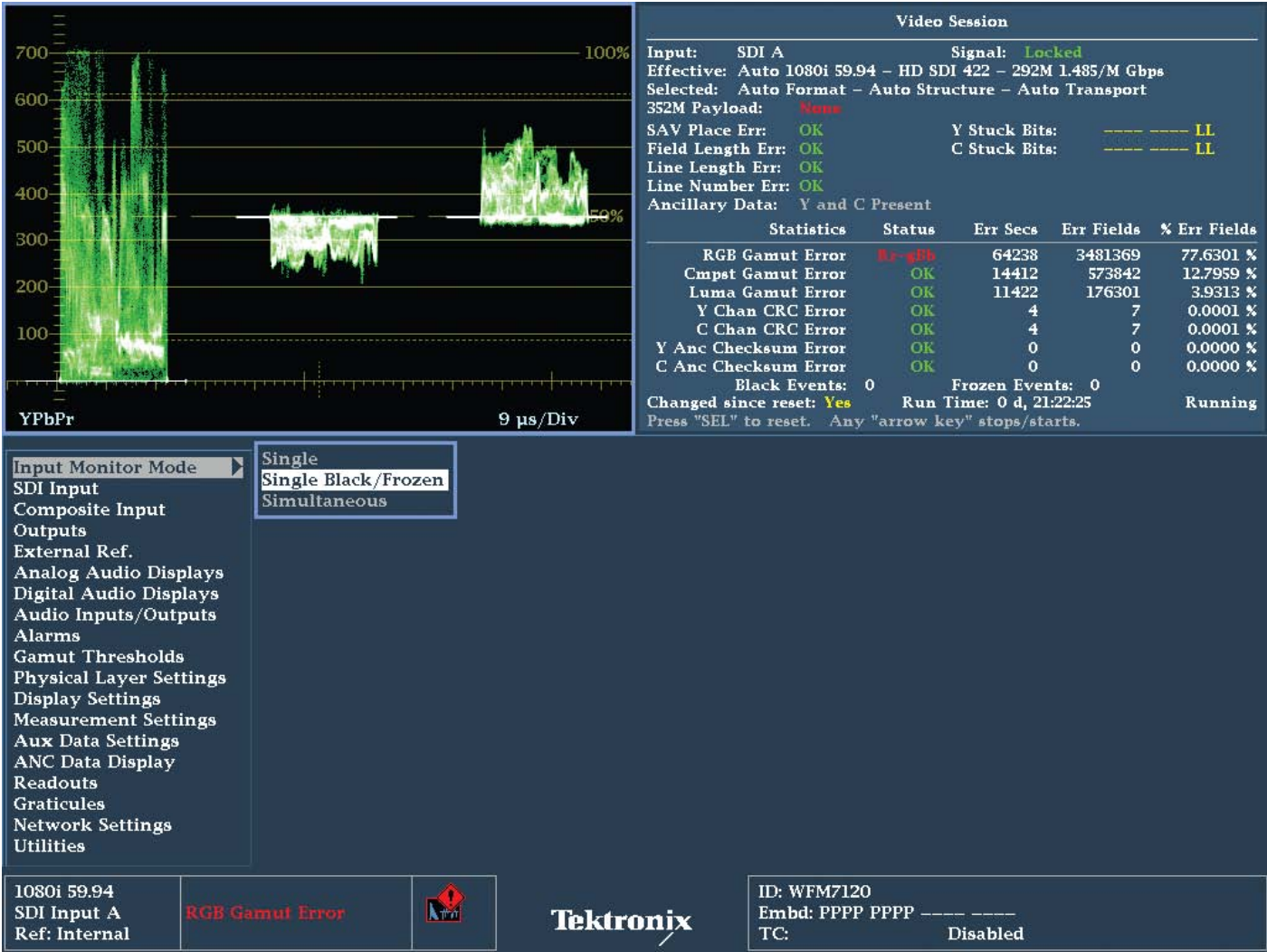
Figure 1. Input Monitor Mode Configuration.
