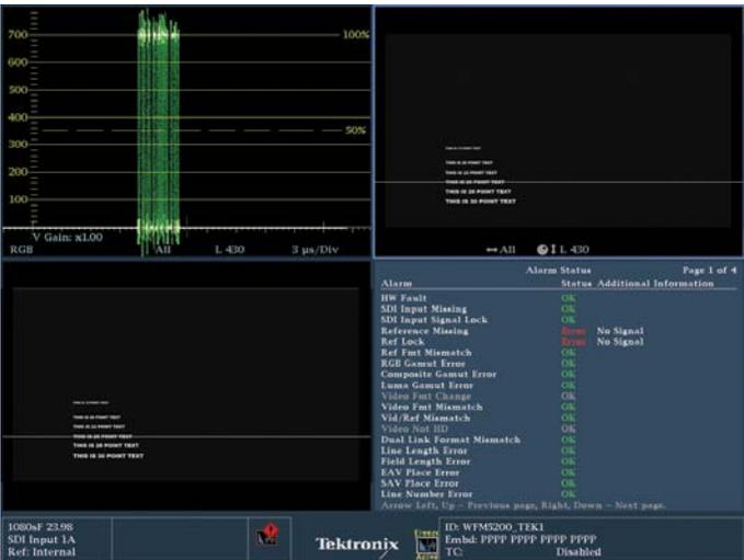
**Figure 20.** Note that when the Line Select is on the text, the waveform shows a strong trace display from top to bottom (upper left quadrant). Also note the Line Select numerical position indicator at the bottom of the picture monitor displaying L430.
