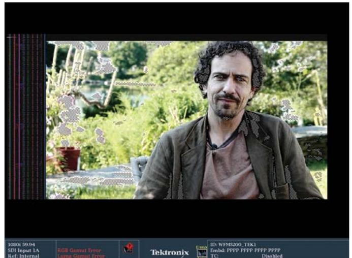
Figure 9. Picture Display showing Brightup indicators where there are gamut errors (both highlights that are too bright and shadows that are too dark. These are indicated by the cross-hatch patterns on the image).
