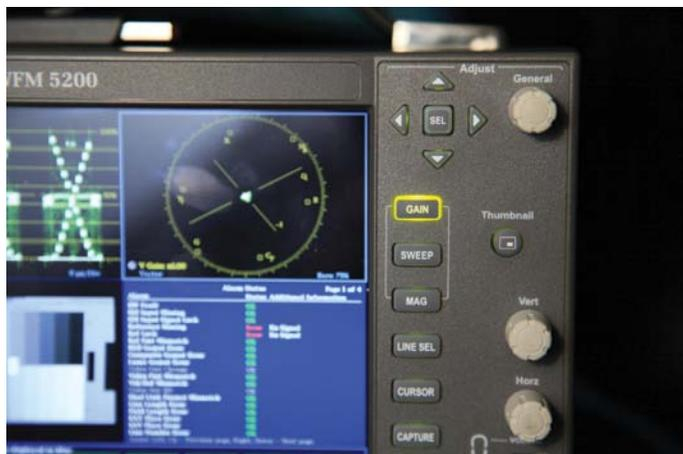
Figure 13. The Line Select button on the front of the WFM5200 is on the right side about half way down.
