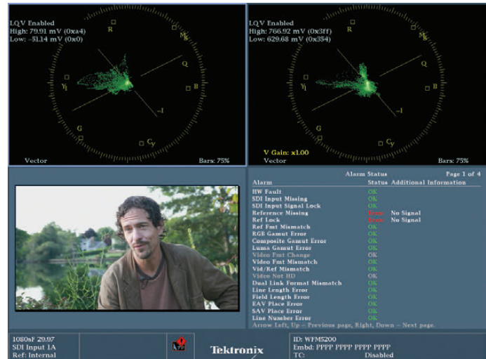
Figure 2-19. The WFM and WVR 5200 are capable of two trace displays. The other two displays must be non-trace displays, like the Picture monitor, Audio bar and Status displays.
