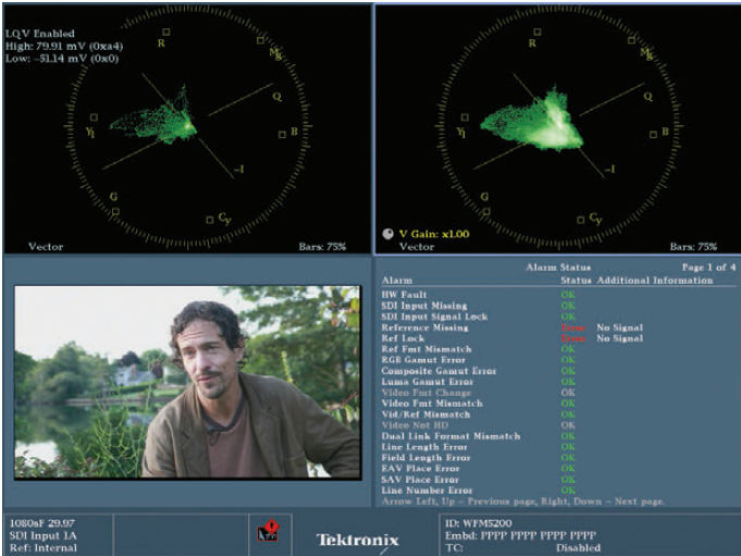
Figure 2-28. A second possible LQV display configuration with one LQV for shadows and one with a standard vectorscope.
