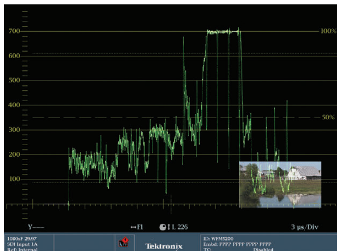
Figure 4-18. Line selection has been enabled. Note the “thinness” of the trace. Also note the thin white line horizontally across the middle of the thumbnail, just below the white face of the barn.
