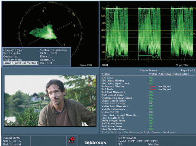
Figure 2-20. Notice the blue selection square around the top quadrant. This shows that the top left quadrant is selected. This selection is done with the Thumbnail or Display Select button.
