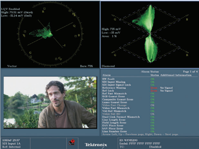
Figure 2-30. A fourth possible LQV display configuration with one LQV for shadows (or highlights) paired with a Diamond Display to monitor gamut violations.
