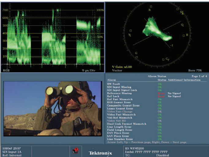
Figure 6-3 One of the most common presets for a colorist would be an RGB Parade waveform monitor matched with a vectorscope. The WFM5200 and WVR5200 can provide two simultaneous “trace” displays, such as the RGB Parade and the vectorscope. The Picture Display and a display like the Alarm Status display are good additions to these two trace displays.
