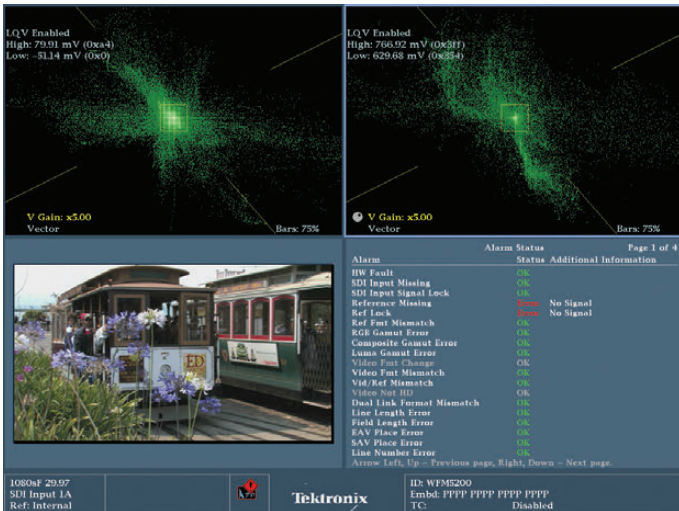
Figure 4-32. This preset for the WFM5200 has two LQV displays. The one on the left is set for the darkest 10% of shadows. The one on the right is set for the brightest 10% of the highlights. Both displays have GAIN set to 2x to focus on the center (black) of the vectorscope, making it easier to dial in the black balance.
