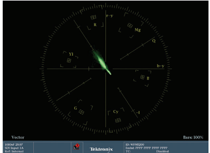
Figure 4-34. This is the vectorscope image representing the footage in the clip of San Francisco Town Hall. Note that the trace extends up the -I line and down towards the blue/cyan targets.
