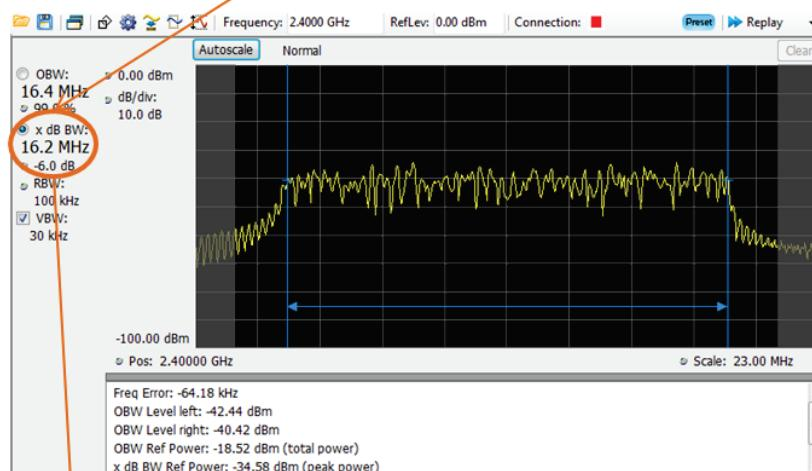
**Step 2:** In the Occupied Bandwidth display, check the -6 dB bandwidth.
