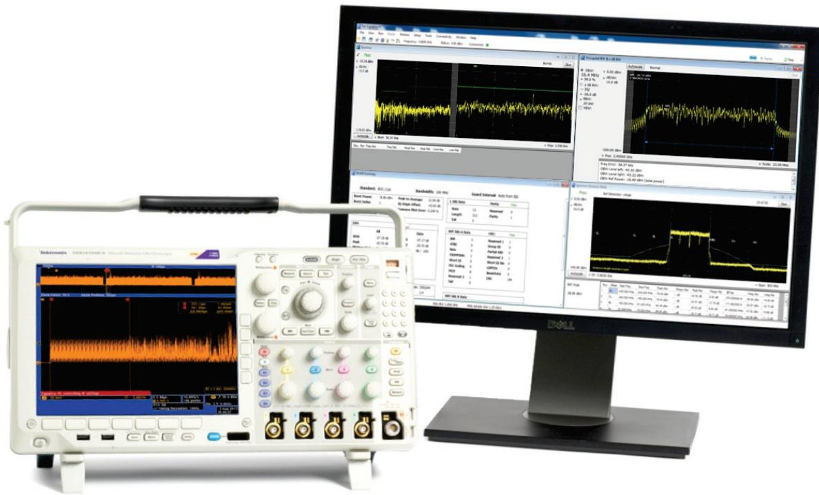
**Figure 3.** Tektronix MDO4000B Paired with SignalVu-PC for Pre-compliance Test
