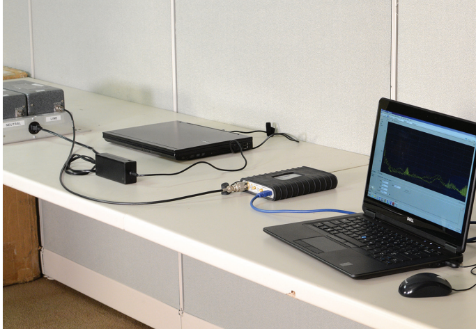
Figure 13. Basic pre-compliance conducted emissions test setup.
