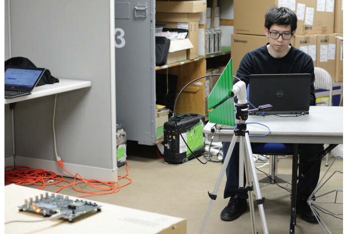
Figure 7. Shows our pre-compliance setup located in a basement of one of our buildings.
