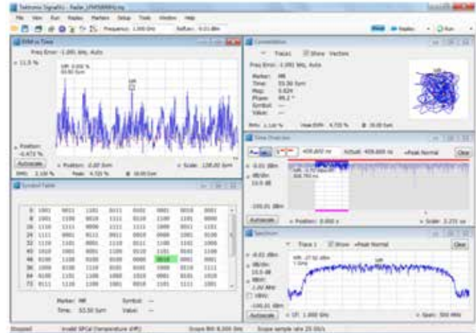
Figure 6. Wideband point-to-point microwave links can be easily demodulated with SignalVu-PC's option SVM. Shown is a 16QAM signal operating at 312.5 Msymbols per second. Note the RMS EVM of less than 3%.
