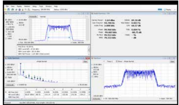
Figure 9. The SignalVu-PC’s suite of powerful measurements and features makes analyzing audio signals efficient and easy. Users can employ audio filtering to affect the results. Multiple measurements, including Occupied Bandwidth, can be easily displayed so the user can monitor a greater number of signal characteristics at the same time. Shown is the same audio waveform as in Figure 8, but filtered with a 3 kHz Low Pass Filter. Audio spectrum is shown in the lower left. Occupied Bandwidth is shown in the upper left.
