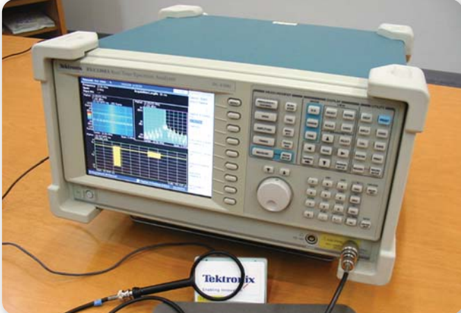
► Figure 1. Example of a setup to test interaction between RFID reader and tag using the RSA3303A and Near Field Probe Set, Tektronix Product number: 119-4146-00
