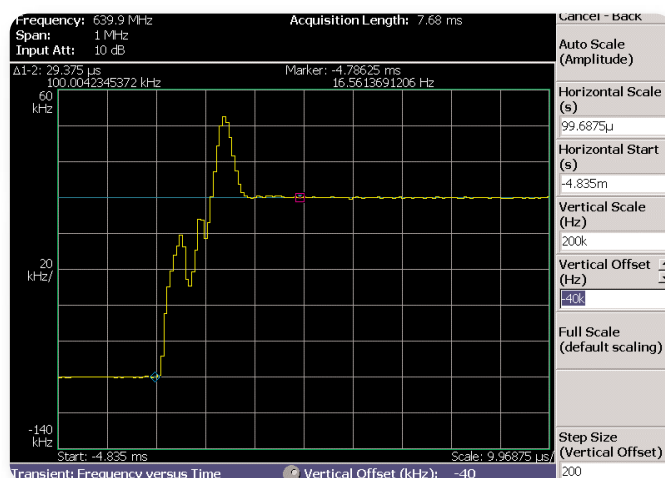
► Figure 6. Switching transient (frequency vs. time) of hopping transmitter shown in Figure 5. Markers show 100 kHz frequency step with transient settling out in 30 \mu sec.
