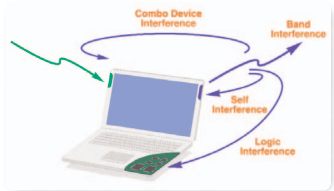
► Figure 3. Modes of combo device interference.
