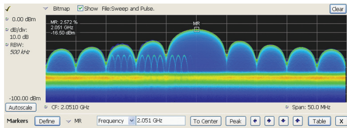
Figure 29. Marker selected to Peak. The reference signal density, frequency, and amplitude are shown on the right hand part of the DPX spectrum display.
