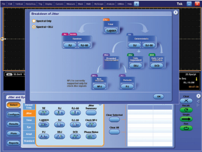
Figure 5. Breaking down jitter into components provides deeper insight. Like NPJ Measurement results that shed light on jitter caused by crosstalk at high frequencies.
