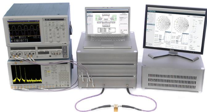
Figure 1. Mesuro's MB Series Open Loop Active Load Pull solution utilizes the unique function and performance of Tektronix equipment for the simultaneous utilization of its waveform measurement and harmonic load pull capability.
