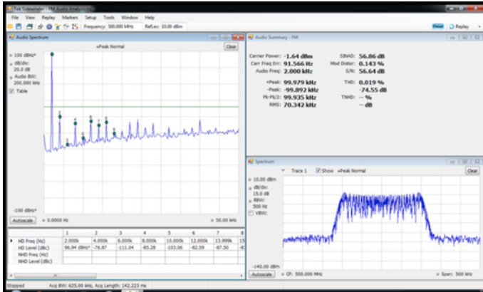
Figure 8. Powerful and convenient modulation and audio measurements are easily produced with RTSAs (Option 10) and SignalVu-PC for oscilloscopes. Shown is an audio waveform captured in “fast frame” mode. RF spectrum is on the right. Audio spectrum measurements are on the left.
